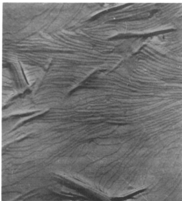
Figure 4 Micrograph of PEO with molecular weight 40 000. Magnification 25 000x
