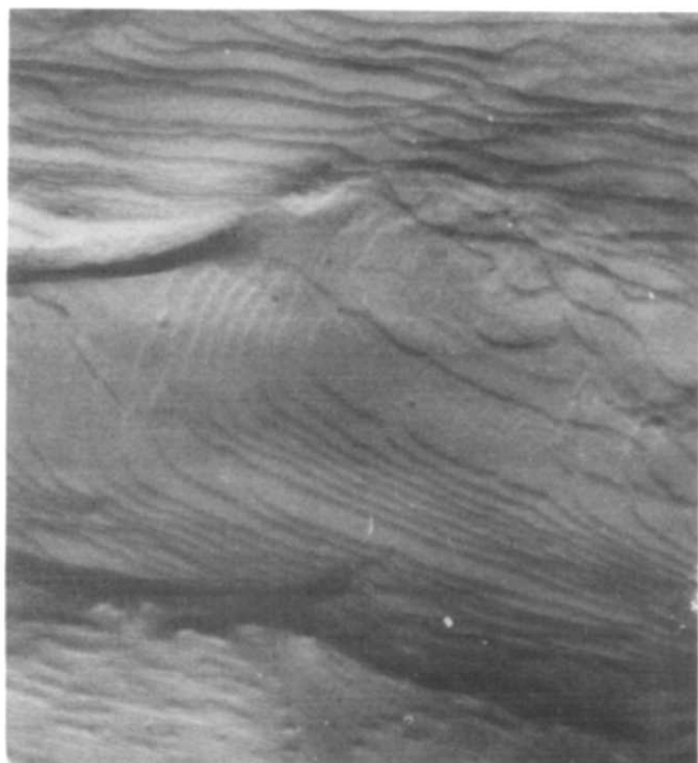
Figure 9 Micrograph of the mixture composed of the MC and PEO-40 000 (point 5 of the phase diagram), magnification 25 000x
