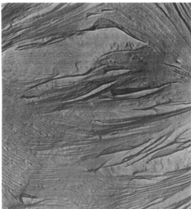
Figure 7 Micrograph of the MC with REO-40 000 in a transmission electron microscope, magnification 25 000x
